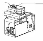
Pressing a sensor switch 2seconds and then sensor light will light once every 2seconds, it represents a sensor working; Pressing a sensor switch 2 seconds again and then a sensor light flash 4 times, it represents a sensor off.
