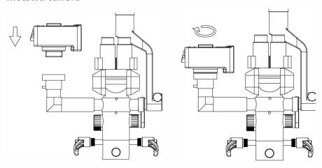
Install a camera to the light splitter tube (Aim at snap points when the camera install to a snap joint and then rotate a camera untill hear a sound of "ka" a camera installation is ok
